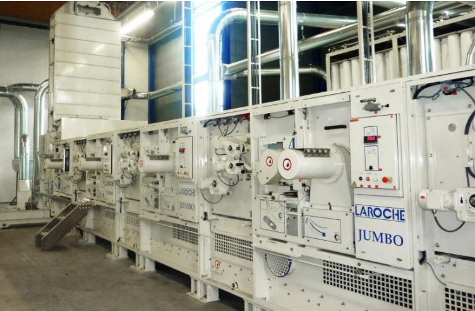
Above: Mechanical textile recycling machine at Frankenhuis. (Photo by Alcon Advies)
