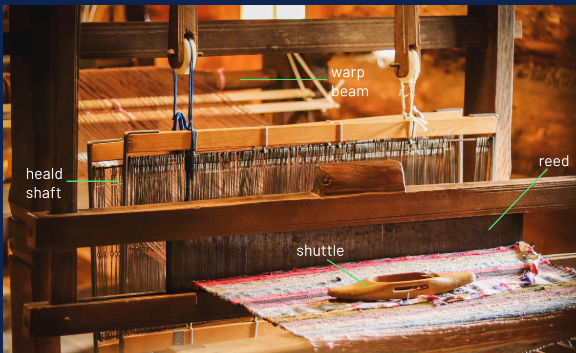
Above: A traditional loom with the warp beam, heald shafts, reed, and shuttle labeled. Photo by Zuzana Kacerová published August, 2019 and was retrieved from Unsplash in June of 2021.
